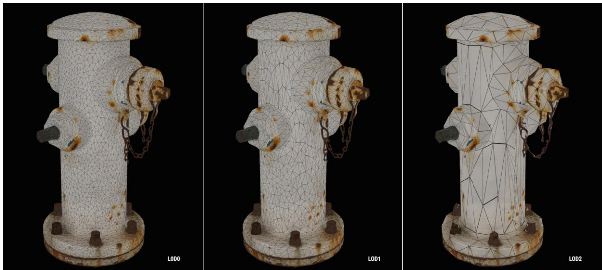
Figure 29 - Asset with different levels of polygonal mesh resolution
